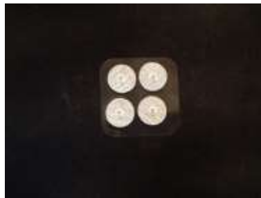
Columbia 700 electrode (.86" diameter)
